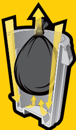
BUILT-IN VENTING CHANNELS
